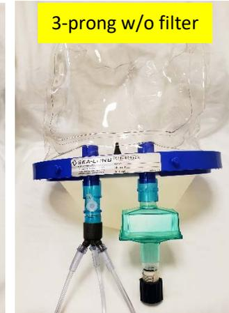
C. 22M adapter, Bact-trap filter, 22MM/15MM adapter, PEEP valve
